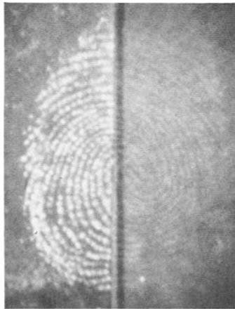
FIG. 3b—As for Fig. 3a, but ninhydrin half (right) treated with zinc. Photographed from VSC-1 using blue-green light and 610-nm filter at room temperature.
